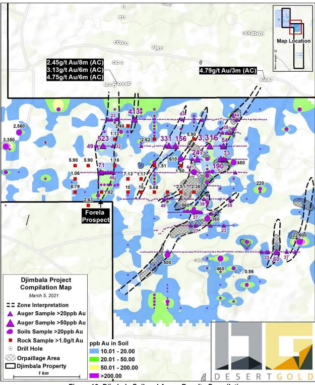
Figure 10: Djimbala Soil and Auger Results Compilation
