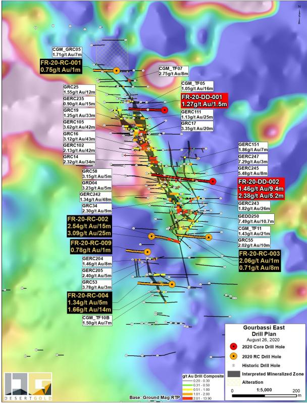
Figure 4. Gourbassi East Drill Plan
