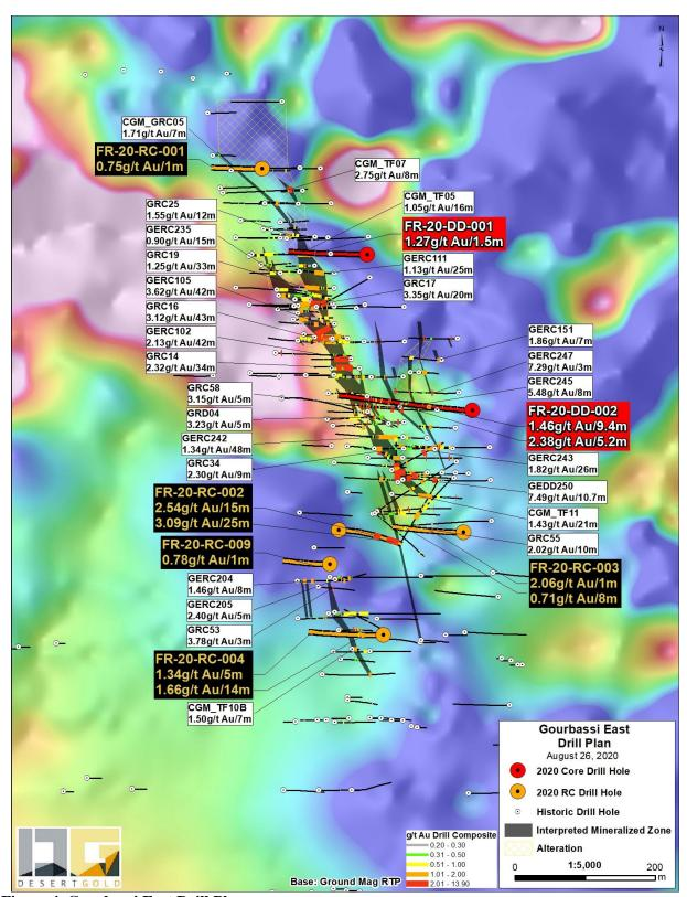
Figure 4. Gourbassi East Drill Plan
