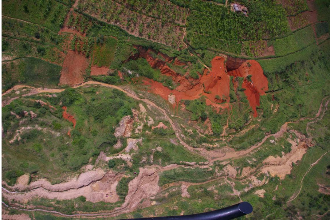
Figure 6.1.1_4 Alluvial Workings, Grey, in Stream, and Large Pit, Byumba, Locality 54 (the pit is stripping overburden from paleo gravels and has been active for over a year)
