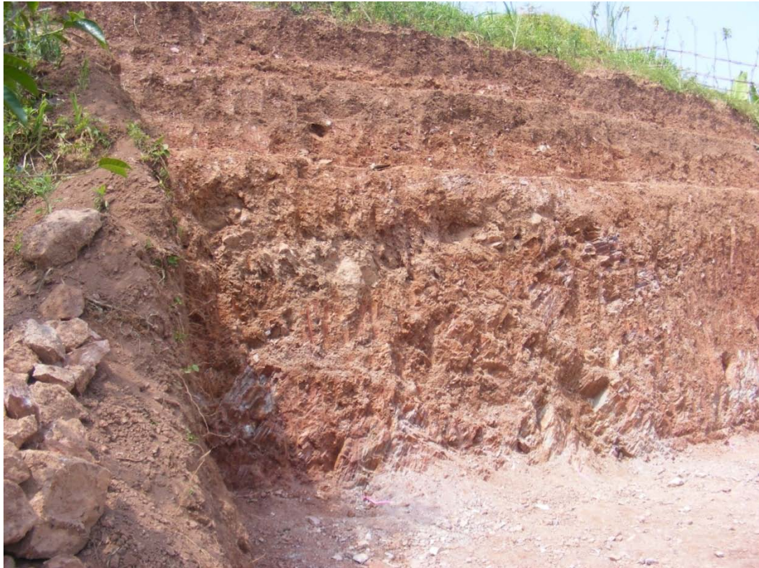
Figure 7.3.1_4 Weathered Phyllite Exposed in the Side of a Drill Pad
